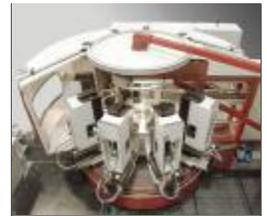
A 10-station rotary transfer machine like this one is part of Remmele Engineering's pilot project
